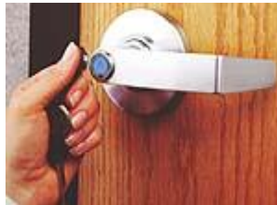
Figure 5.14 - The In/Out board iButton reader
